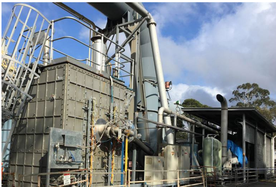
Figure 3.6 Trial of CSIRO's VAMMIT technology at Appin Coal Mine
